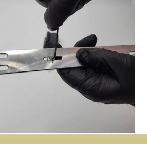
Use a machinist square or carpentry triangle to make sure the last D part is 90 degrees to the part B. Keep it approximately in the middle of the pocket. Tighten until fingertight, then a 1/8 turn.
