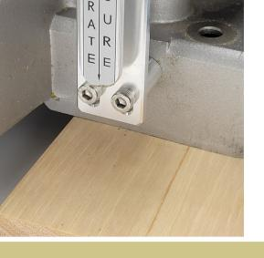
The pockets were machined to allow variations in planers. The bolts can be anywhere within the pocket, but they should not be rubbing against the very ends of pockets. If they are, adjust this from opposite side.
